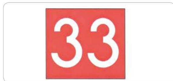
[그림 2-26] Holding Position Sign at Beginning of Takeoff Runway
