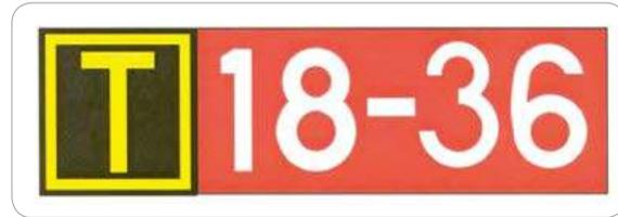
[그림 2-32] Taxiway Location Sign Collocated with Runway Holding Position Sign
