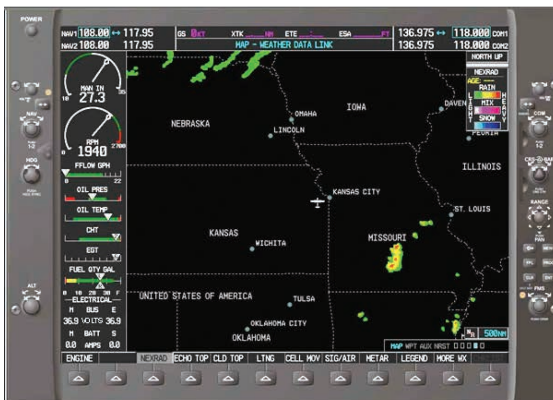
Figure 13-18. NEXRAD radar display (500 mile range). The individual color gradients can be easily discerned and interpreted via the legend in the upper right corner of the screen. Additional information can be gained by pressing the LEGEND soft key, which displays the legend page.
