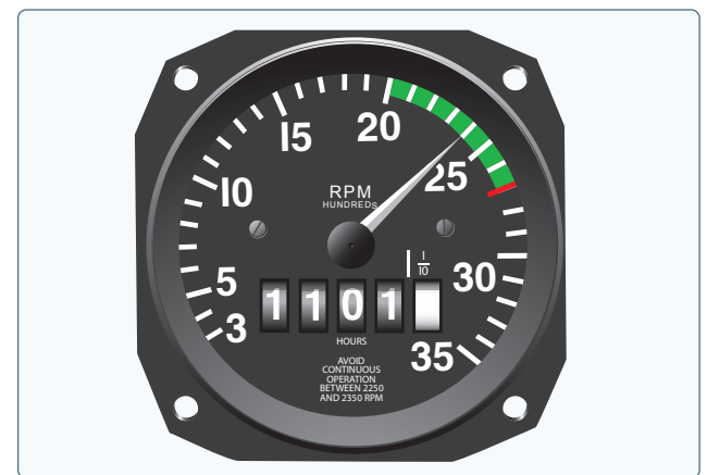
Figure 7-8. Engine rpm is indicated on the tachometer.
