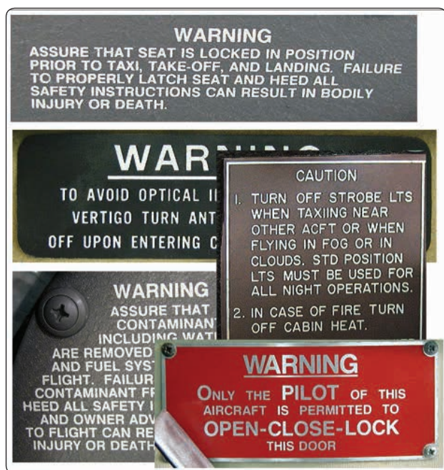
Figure 9-5. Placards are used to depict aircraft limitations.
