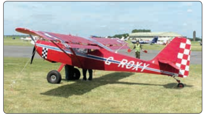
Figure 6-9. Flaperons on a Skystar Kitfox MK 7.
